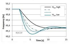
By adding inertia, stability can be increased
