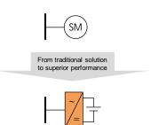
A proposal from ENTSOe is that almost all grid connected generators must behave like a synchronous generator (inertia and overload capability)
