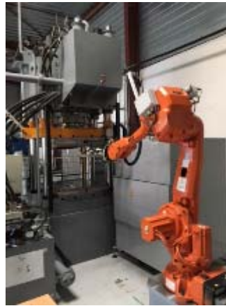
Robotized stamping press
